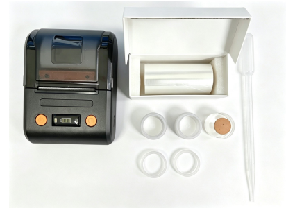
SAMPLE PREP KIT — PRINTER, MYLAR FILM, SAMPLE CUPS & PIPETTE
